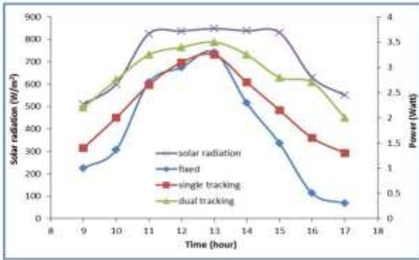
Figure (11): Relation between solar radiation and power with time.
