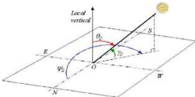
Figure (1): The various angles and other important parameters describing the position of the sun in the sky viewed from an observer O.
