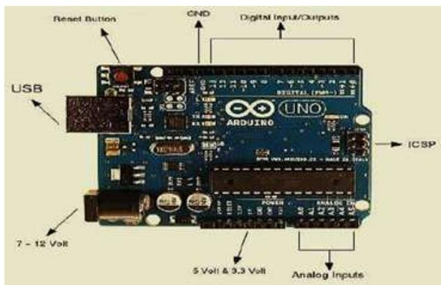
Figure (6): Arduino and its components
