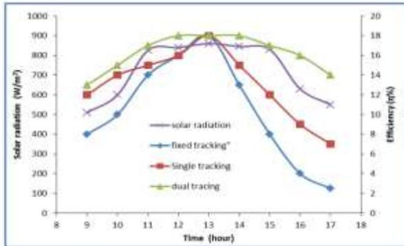
Figure (12): Relation between solar radiation and efficiency power with time.
