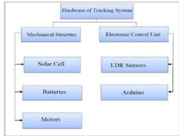
Figure (4): Block diagram of the tracking system.
