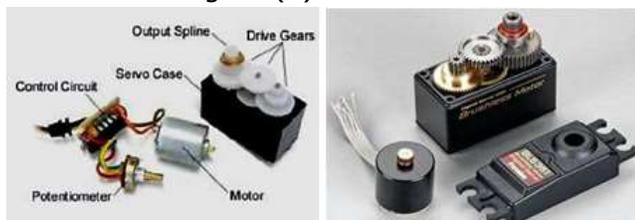
Figure (7): Servo motor used in the present work with its accessories.
