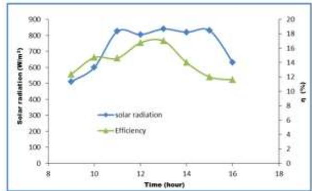
Figure (10): Relation between solar radiation and Efficiency with time.
