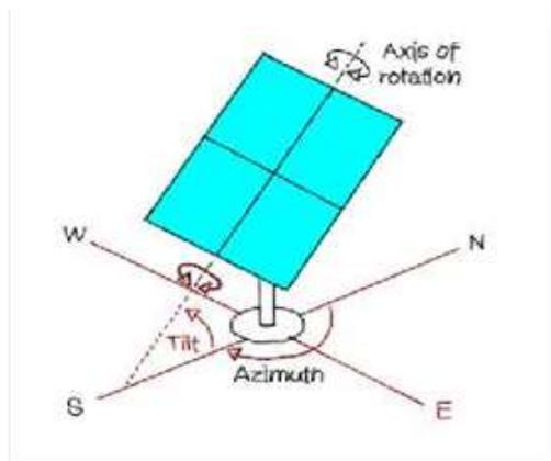
Figure (3): Dual axis geometries [18].
